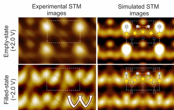
The further support for the model with the inner dimer was gained from the comparison of the experimental high-resolution STM images with the simulated ones.
