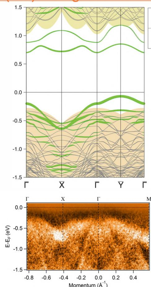
The electronic band structure calculated for the Si(100)2×3-Ag reconstruction model with the inner Si dimer and experimental data obtained by using ARPES technique. One can clearly see that it is semiconducting with an indirect band gap of ~ 0.8 eV.
