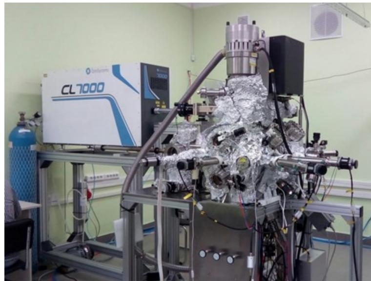
Fig. 3. Experimental vacuum system for the MAX-materials synthesis
