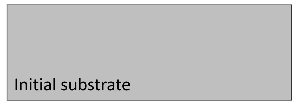
p-type monocrystalline silicon wafer of (100) orientation and 12 Ohm·cm resistivity
