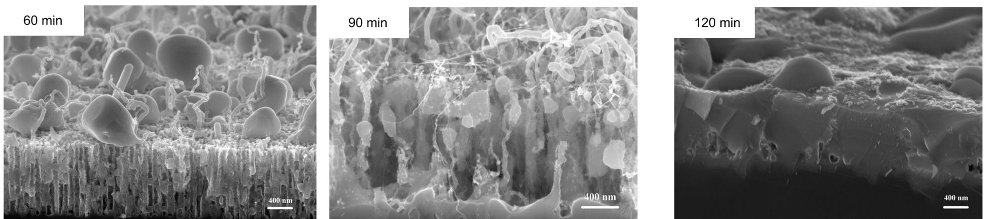
Fig. 4. SEM images of silicon-germanium nanocomposite after thermal annealing for different time at 950°C in argon.
