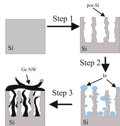
Fig.1 Schematic illustration of Silicon-Germanium nanocomposite fabrication
