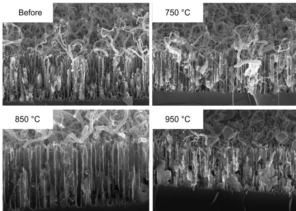
Fig. 2. Scanning electron microscope (SEM) images of silicon-germanium nanocomposite before and after thermal annealing at different temperatures for 10 min in argon.
