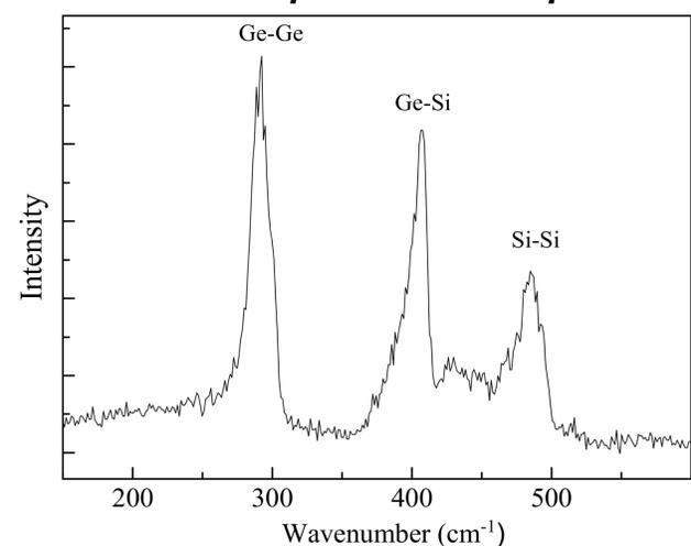
Fig. 3. Raman spectra for sample after thermal annealing for 120 min at 950°C.
