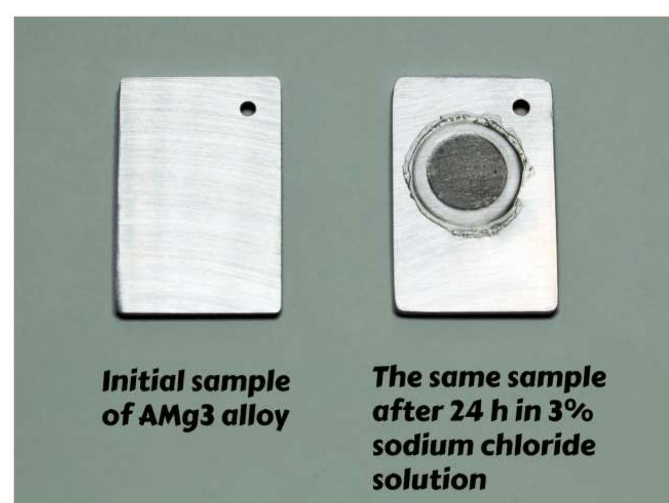
Figure 1 — Corrosion of the AMg3 alloy in the aggressive environment
