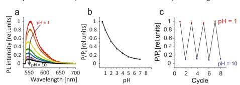
(a) a series of PL spectra of the pH sensitive laser-textured surface upon successive acidification of the surrounding solution; (b) change in signal intensity upon cyclic filling of the microfluidic cell with basic (pH = 10) and acidic (pH = 1) solutions; (c) change in signal intensity upon cyclic filling of the microfluidic cell with basic (pH = 10) and acidic (pH = 1) solutions. dependence of the normalized PL intensity P/P₀ on pH value.
