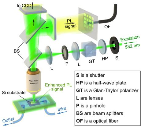
Experimental setup for PL measurements and pH sensing tests.
