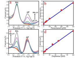
Cyclic voltammograms (CVs) of Nibased electrode recorded in solutions containing dopamine (blue) and acetaminophen (green) individually and as a mixture (red). The amperometric current of the fabricated Ni-based electrode recorded in the presence of different concentration of dopamine (b) and acetaminophen (c).
