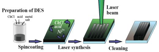
We performed the deposition of nickel on substrate with DES mounted in a vertical position using the experimental set-up with continuous wave 532 nm diode-pumped solid state Nd: YAG laser was used. The amount of the components used for preparation of DES was:
