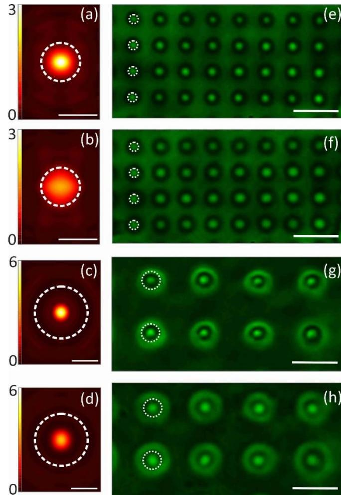
(a, e) 1  $\mu\text{m}$  hemisphere, gap 0.2  $\mu\text{m}$
