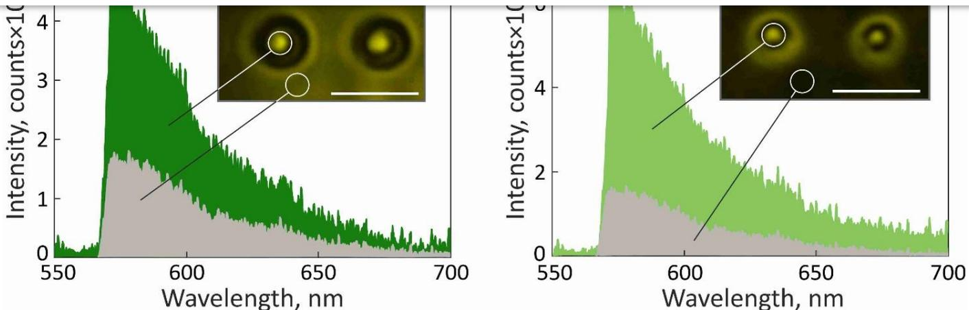
(a) 1 $\mu\text{m}$  hemisphere, gap 0  $\mu\text{m}$ ; (b) 1 $\mu\text{m}$  hemisphere, gap 0.2  $\mu\text{m}$ ;
