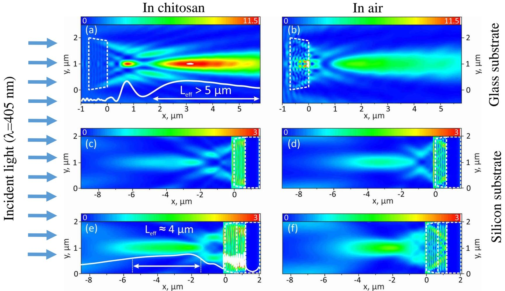
Once the microstructure is placed at a certain distance from the substrate it is possible to obtain **PNJ in reflection mode without standing wave modulation!**
