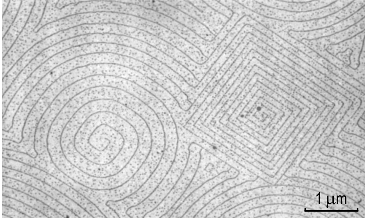
Fig. 10.20. Step structure at the emergence points of screw dislocations produced by sublimation of an NaCl crystal at 400°C for 90 min in a high vacuum (after Krohn and Bethge [10.12])
