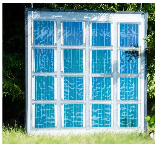
Fig. 1. Photo-image of the fabricated perovskite solar panel (16 modules).
